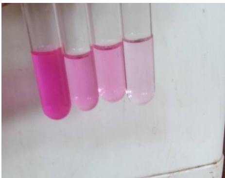
Figure 4 d Photograph of degradation of Rhodamine B dye with Zn_{0.98}La_{0.01}Ce_{0.01}O as catalyst
